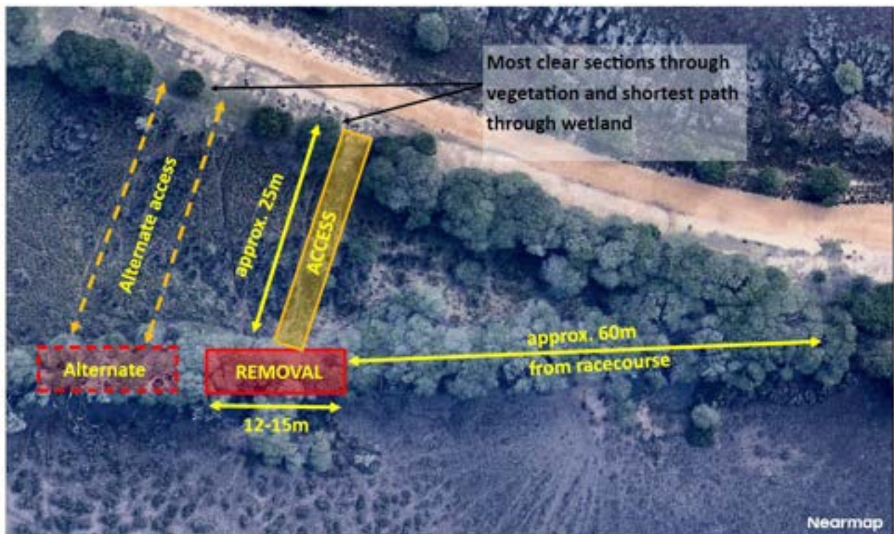
Figure 3-3 Proposed levee works
