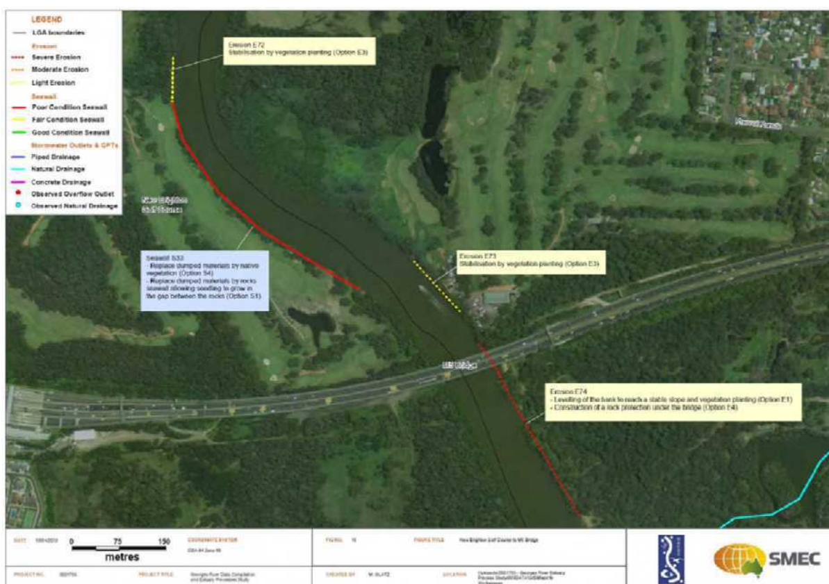
Figure 7 Example of foreshore erosion and structure condition assessment undertaken as part of the Georges River Estuary Processes survey (source: SMEC, 2010).
